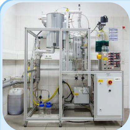
continuously tube reactor
