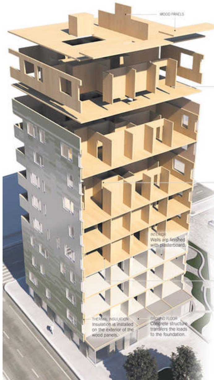
**Cross-Laminated Timber (CLT)** is gaining a significant popularity among structural products as a **sustainable alternative to steel and concrete**. CLT has a **low carbon footprint** and provides **comfortable living conditions**; moreover, the high strength-to-weight ratio, the prefabrication process and the erection speed are additional key points of its broad diffusion.
