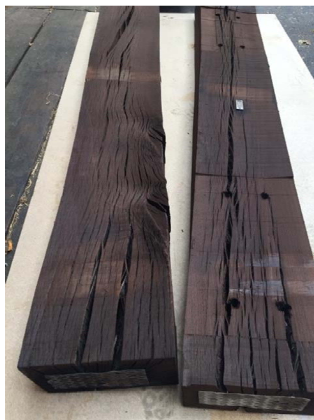
Figure 5: impregnated sleepers before (left) and after (right) thermo-treatment]
