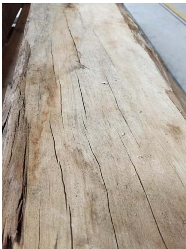
Figure 4: sleeper before impregnation
