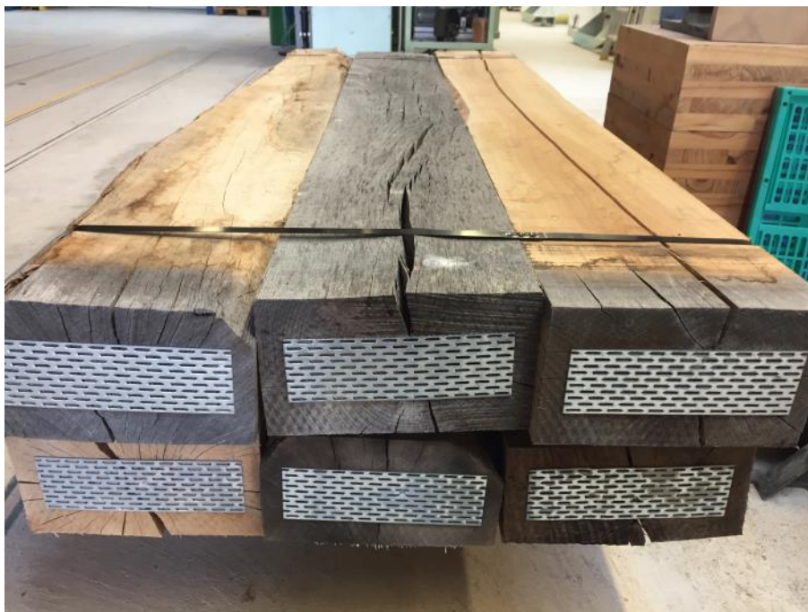
Figure 3: sleepers before impregnation
