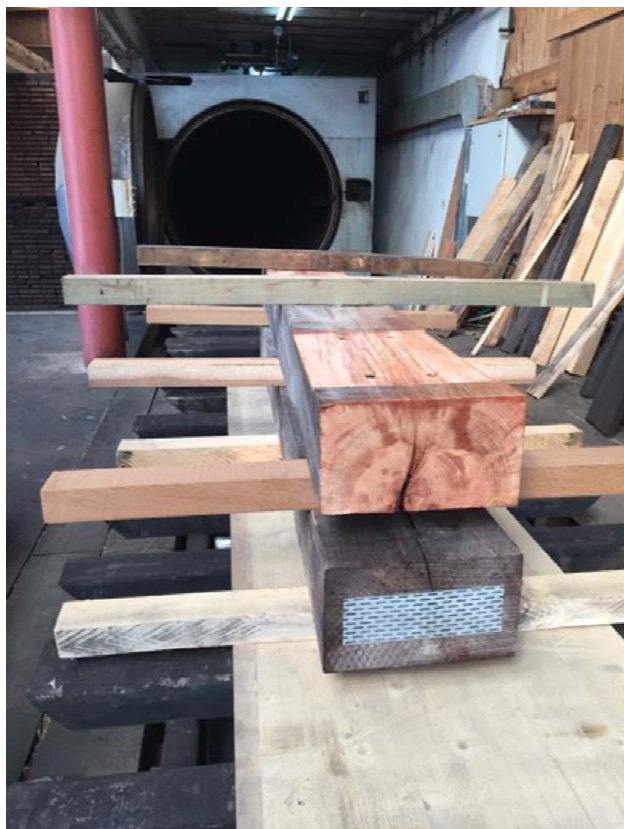
Figure 5: impregnated sleepers before (left) and after (right) thermo-treatment]
