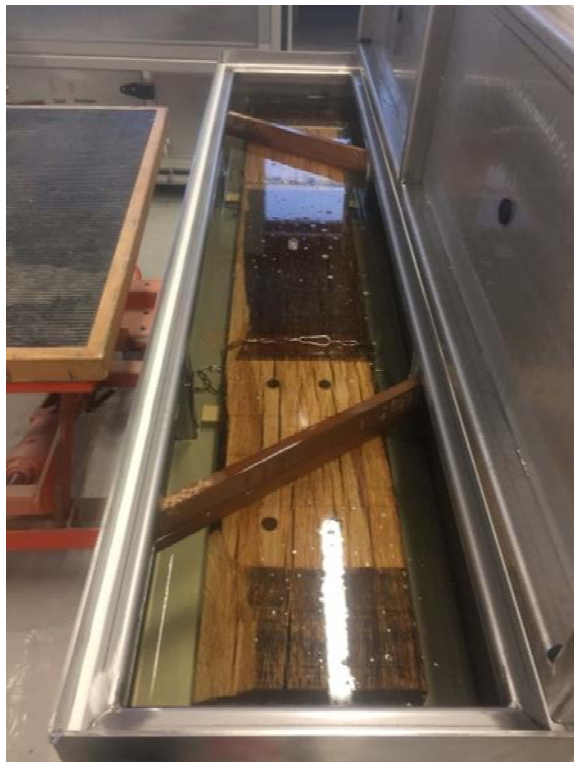
Figure 2: oak sleeper soaked into lactic acid
