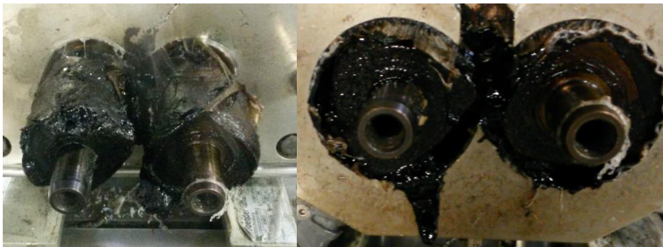
Figure 5: Thermal degradation during compounding of CA/GTA with acetylated hemicellulose in the internal mixer
