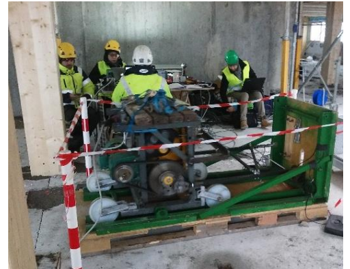
Figure. Structure of the building Treed-It in Paris, designed by Vinci Engineering with Arbonis as main contractor of the timber parts, and a photo from the full-scale measurements with CSTBs shaker in operation in the building.
