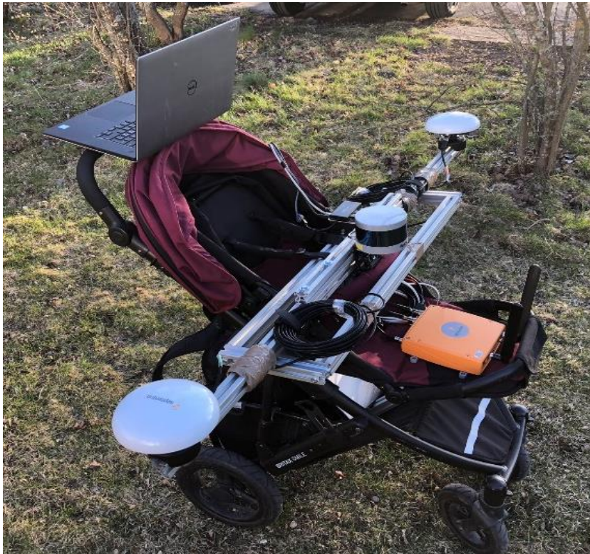
AVATAR sensor equipment mounted on a stroller (NIBIO)
