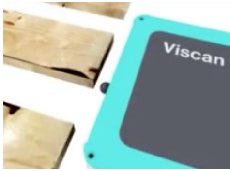
MOEdyn (ViScan) of dried boards: At Sävar Sawmill and Derome Sawmill x2
