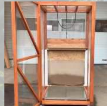
Figure 3: Decay module in the CLICKdesign tool the splashwater test rig (University Göttingen)
