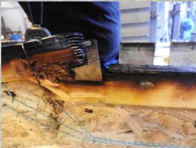
Figure 1: Finger joint of I-joist failed in adhesive (RISE)
