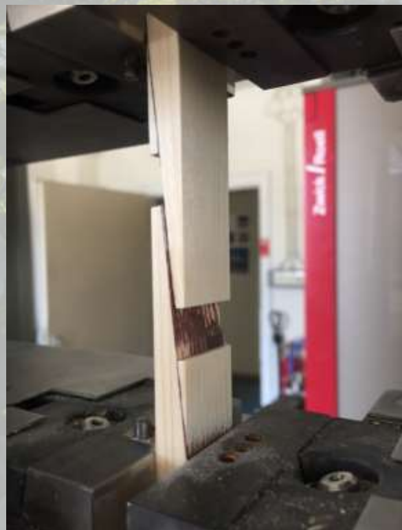
Figure 5: TETT test specimen tested at ambient temperature (20°C) (MPA Stuttgart).
