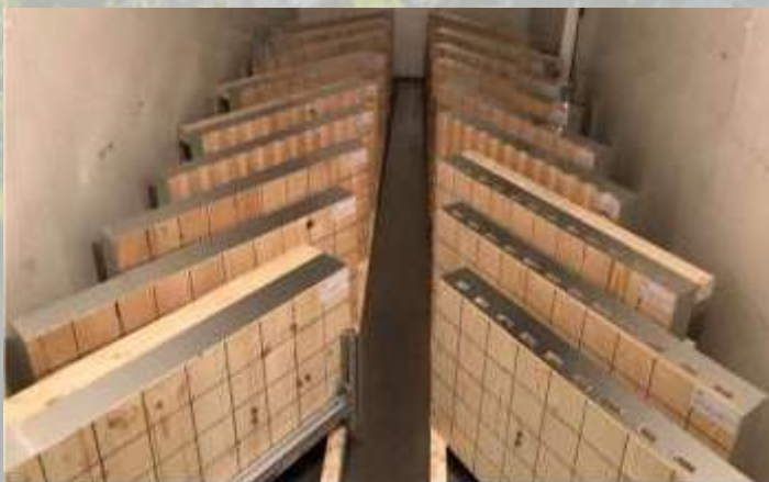
Figure 5: Multifunctional CLT elements under climatic testing in the climate chamber (TUM)
