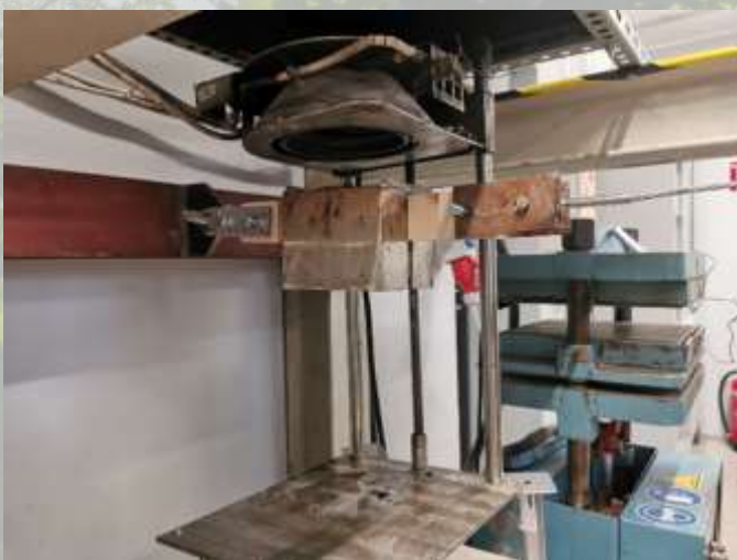
Figure 3 and 4: Loaded cone heater method for Finger joints (RISE/TALTECT).
