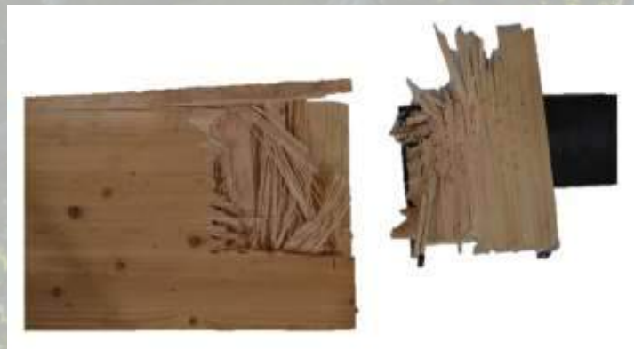
Figure 4: Experimental investigation of brittle failure in CLT connections (ZAG)
