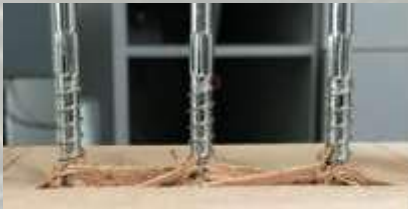
Figure 1: Row shear failure mode of a group of three axially loaded screws. (Karlsruhe Institute of Technology, LERMAB Epinal and Technical University of Graz ).
