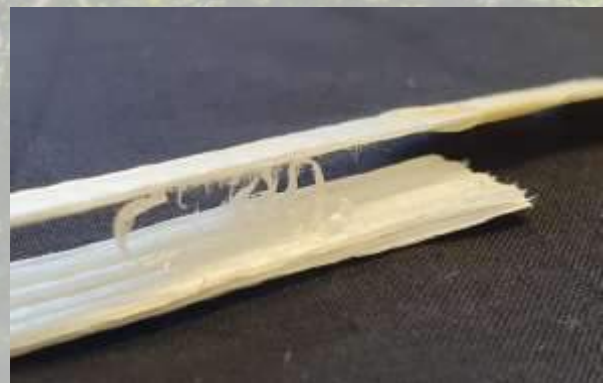
Figure 2: A lap shear sample prepared with delignified spruce veneer and recombinant spider silk protein. (Jennifer Teerstegen)
