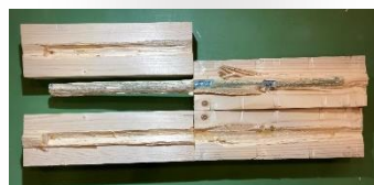
Figure 3. Adhesive failure in finger jointed specimen © FIRENWOOD
