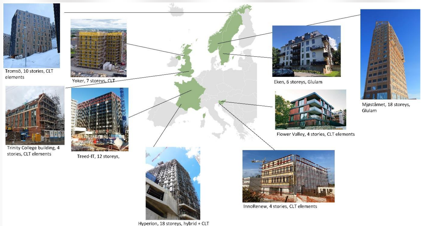
Figure 17. Buildings tested with full-scale forced vibrations within the project (© Marie Johansson; DynaTTB Project)
