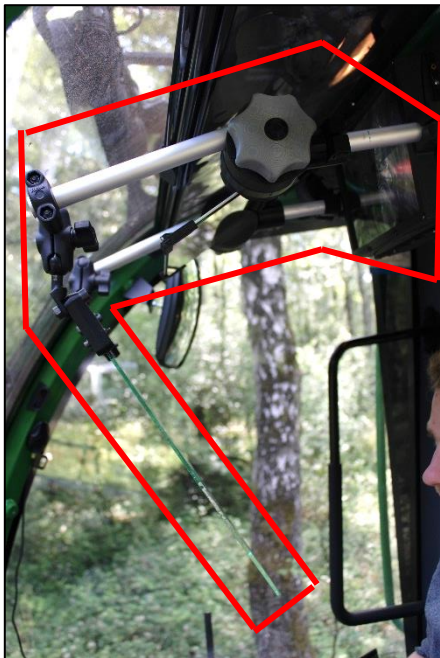
Head-up display in John Deere Harvester during harvesting operation and display content provided by the LiDAR.
