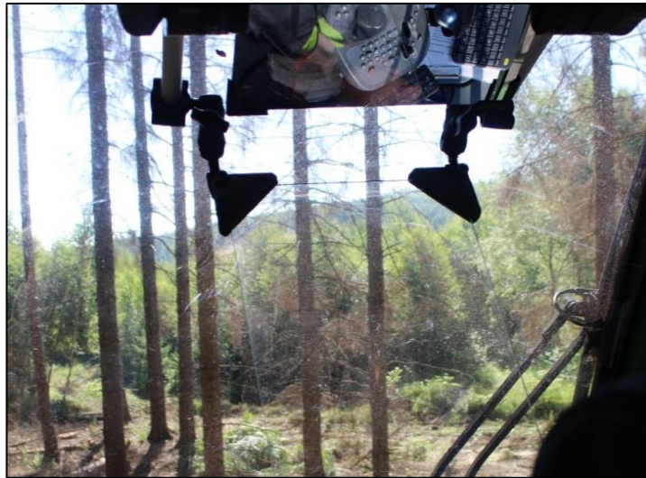
Head-up display in John Deere Harvester during harvesting operation and display content provided by the LiDAR.
