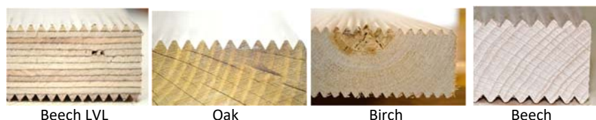
Figure 1: Shallow grooves on the surface of hardwood specimens.
