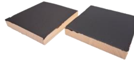
Spruce wood coated with polyphenols and biochar
