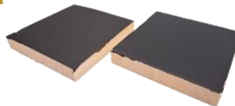
Spruce wood coated with polyphenols and biochar
